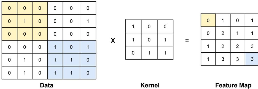
Figure 6: Simplified Example of 2D Convolution
