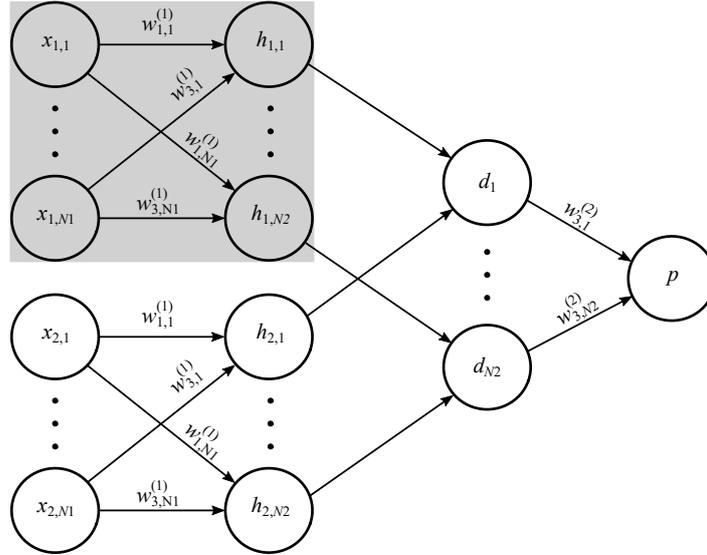
Figure 8: Example of a SNN with two twin networks, with network 1 highlighted in the figure with a gray shaded region. The features extracted by the twin networks in the hidden layers ( $h_{i,j}$ ) have their similarity calculated in a common layer ( $d_j$ ). Finally, the node  $p$  represents a logistic likelihood function. Adapted from [KZS15]
