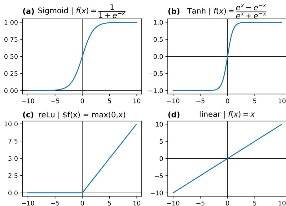
Figure 4: Activation Functions: (a) Sigmoid; (b) Hyperbolic Tangent (Tanh); (c) Rectified Linear (ReLU - Rectified Linear Unit) and; (d) Linear.
