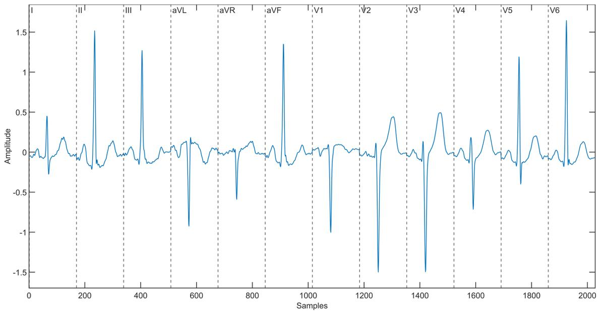
Figure 11: ECG signal with the 12 leads concatenated
