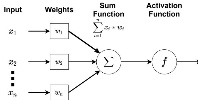
Figure 3: Example of a neuron with  $n$  inputs.
