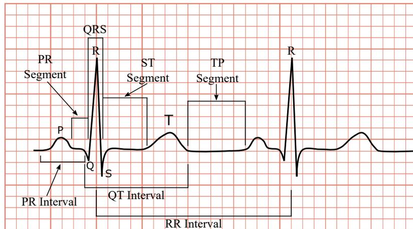
Figure 1: Main components, segments and intervals of an ECG signal.
