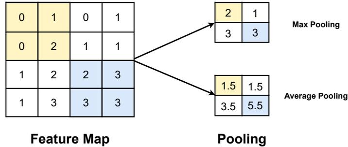
Figure 7: Example of pooling with stride 2
